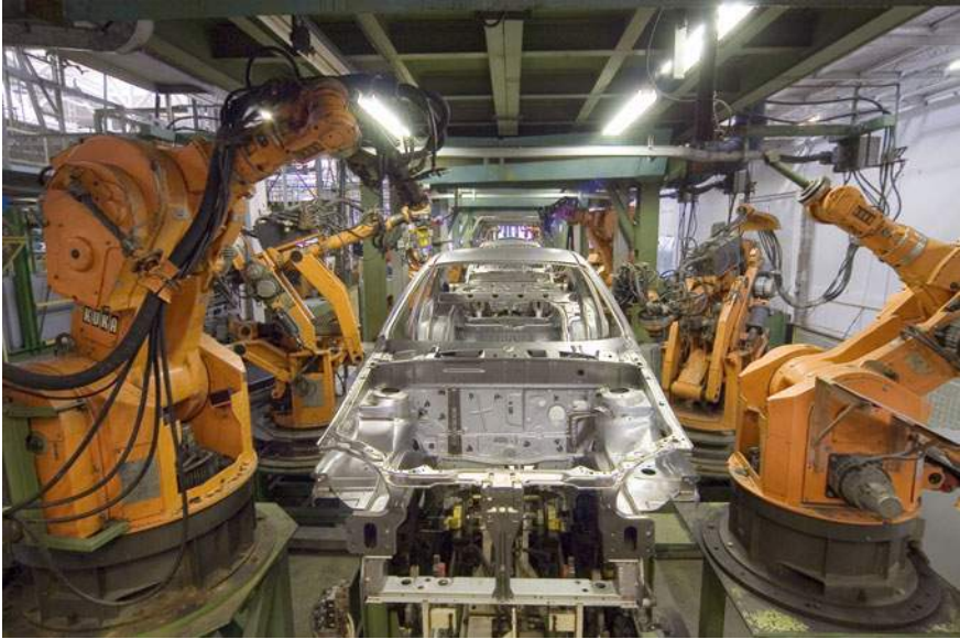
Fig. 1.3 Robots on an assembly line in a car factory. Source https://commons.wikimedia.org/wiki/File:AKUKA_Industrial_Robots_IR.jpg by Mixabest (Own work). CC BY-SA 3.0 ( http://creativecommons.org/licenses/by-sa/3.0 ) or GFDL ( http://www.gnu.org/copyleft/fdl.html ), via Wikimedia Commons
