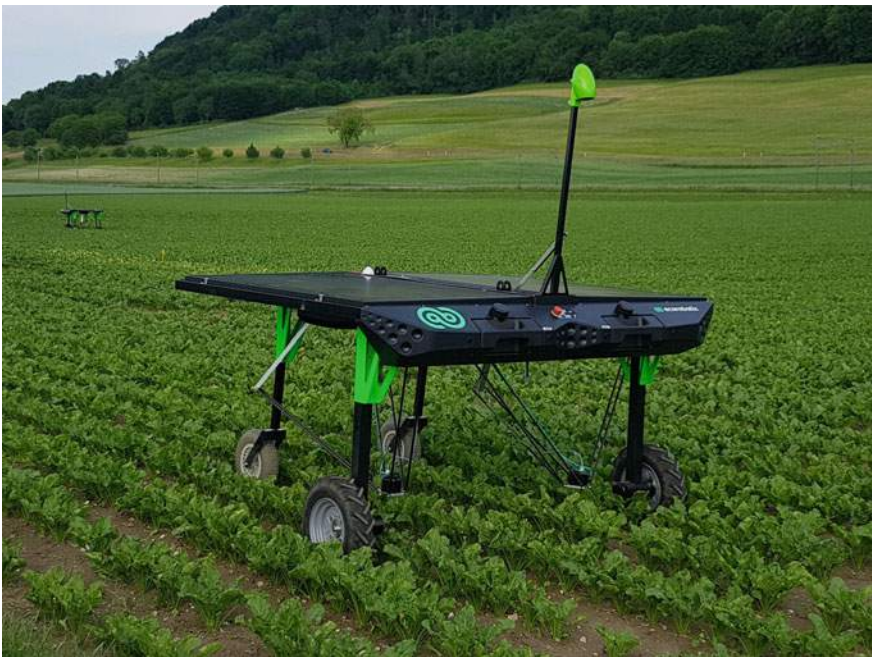
Fig. 1.4 Autonomous mobile robot weeding a field (Courtesy of Ecorobotix)
