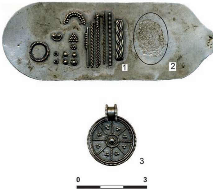
Fig. 13. An examples of soldering filigree and granulation with chemical solder: 1 – decorative elements of filigree and granulation occurring on the analyzed finds; 2 – the porous surface of the silver plaque as the result of a shallow diffusion chemical solder based on copper compounds; 3 – an example experimentally made a silver pendant in filigree and granulation technique soldered with chemical solder (according to M. Sekuła, photo M. Natuniewicz-Sekuła)
