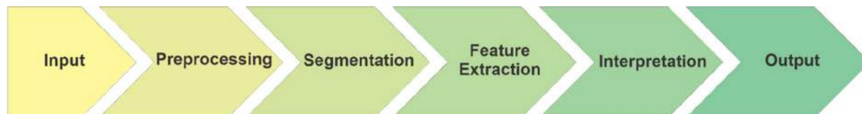
Figure 30 -- The Machine Vision Image Processing Process
