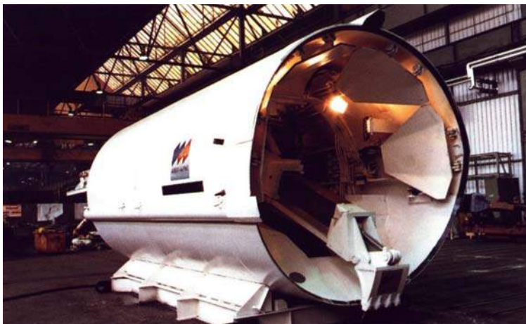
Fig. K-2. Shield support with face plates (visible middle left turned into the machine) and ripper-loading device
