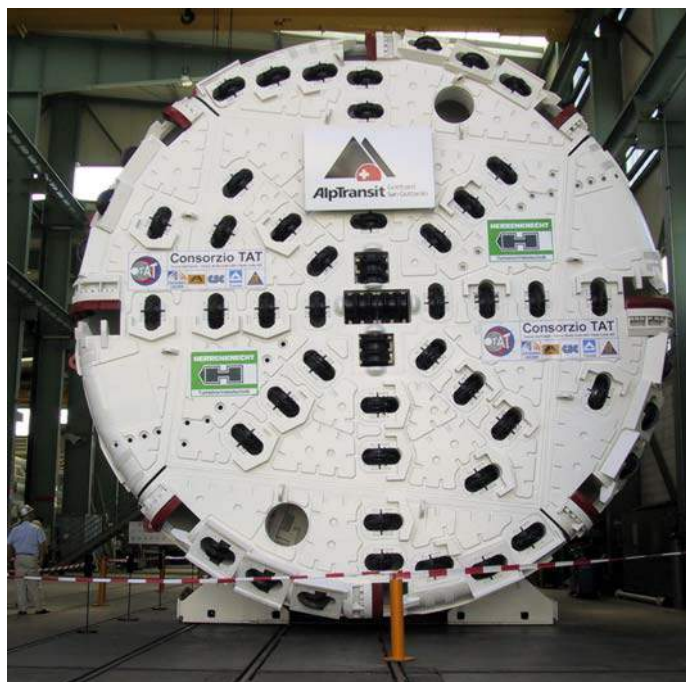
Fig. I-3. TBM cutting wheel with disk cutters. Diameter 8.89 m. St Gotthard tunnel (photo: © AlpTransit, AlpTransit, 2002)
