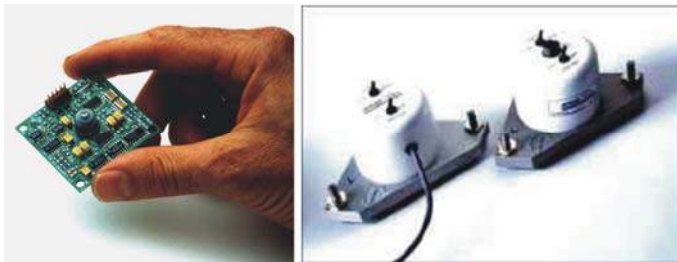
Fig. L-5. Tilt meter (photos: Applied Geomechanics Inc., 2003)
