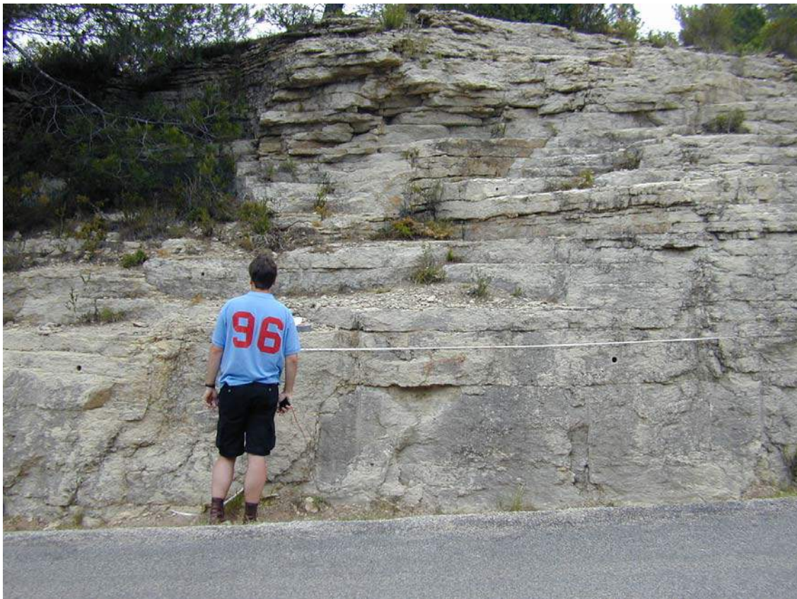
Fig. E-1. Decrease of bedding spacing (“bankink” spacing) nearer to the original surface due to weathering (photo Verwaal, 2001)
