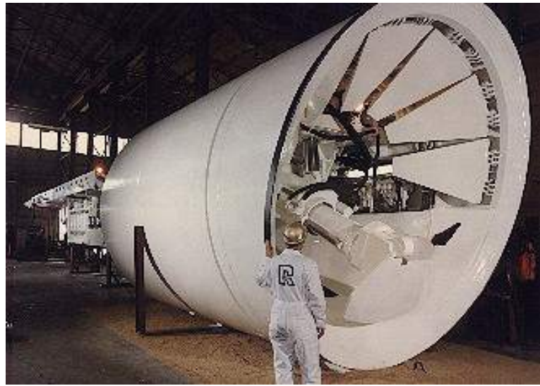
Fig. J-5. Digger shield. The ground moves into the shield under its own pressure. The extraction of the ground from the shield controls the progress. Permanent support is installed behind the shield (photo. Traylor)
