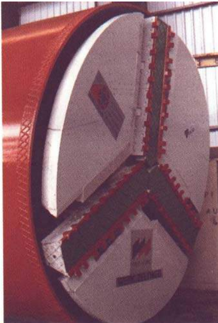
Fig. K-4. Cutting wheel for non-cohesive or low cohesive soft ground (soil) (after Voest-Alpine Bergtechnik, Austria)
