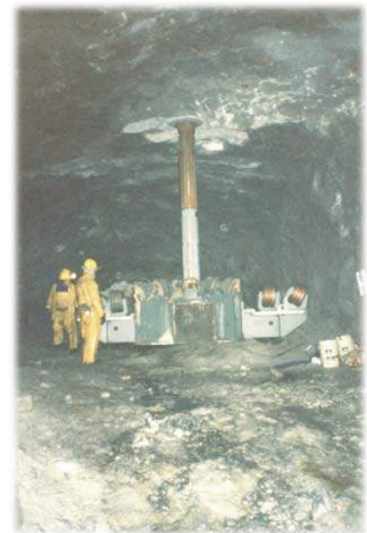
4.3 m Reamer at Cameco's Eagle Point Mine, Saskatchewan, Canada
