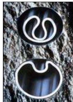
Fig. J-11. Swellex ® rock bolt. Top installation before expanding, below: after expanding due to water pressure (after Atlas Copco, 2002)
