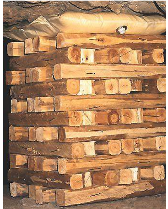
Fig. J-22 Timber pack (An APOLLO modular pack installed with PACKSETTER Non-Weeping pre-stressing) (photo: MONDI TIMBER)
