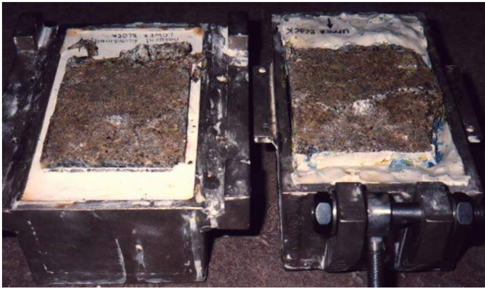
Fig. C-18. Prepared sample for shear box test. The sample halves are imbedded in cement. Test direction is in the length direction of the sample. (after Baardman, 1993)
