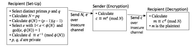
The following is an example to illustrate how RSA encryption and decryption works.
