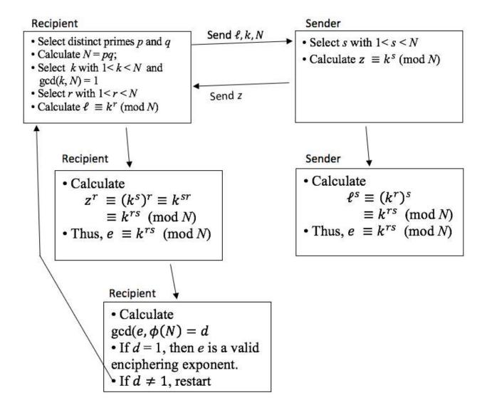
The following is an example to illustrate how the Diffie-Hellman key exchange works.
