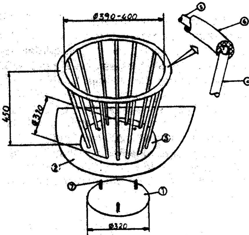
ALTERNATIVE FIXING METHOD FOR BASKET IS TO HAVE A HOLE IN THE BOTTOM OF THE BASKET. THE BASKET IS THEN FIXED TO A PERMANENT THREAD IN THE POOL BOTTOM. THIS FIXING METHOD GUARANTEES THAT THE BASKET STAYS IN POSITION.
