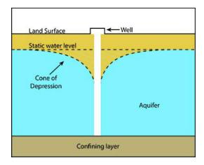
The amount of water that can be removed from an aquifer is its **specific yield**. Specific yield is a percent, and is based off of the material the aquifer is made of. Here is a table for typical rock/soils.
