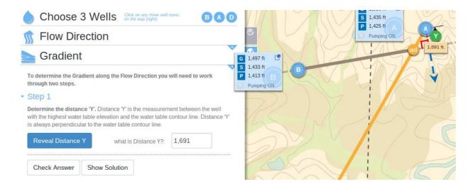
Now time to find the hydraulic gradient, i. Take the change in elevation from A to B, and divide by Y, to get the gradient.
