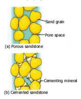
This picture helps explain groundwater flow. In the porous sandstone, water can move freely, as it can easily move around the sandstone particles; it could be an aquifer. But in the cemented sandstone, water flow is blocked, and cannot flow freely; it would be an aquitard.
