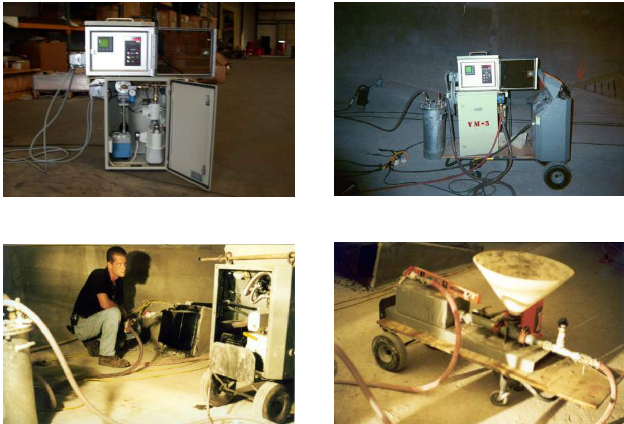
Figure 4.2 - Vacuum Grouting Equipment, Digital Volumeter (up (upper left), Void Volume Measurement (upper right), Grout Pump (lower left), Vacuum Grout injection (lower right)
