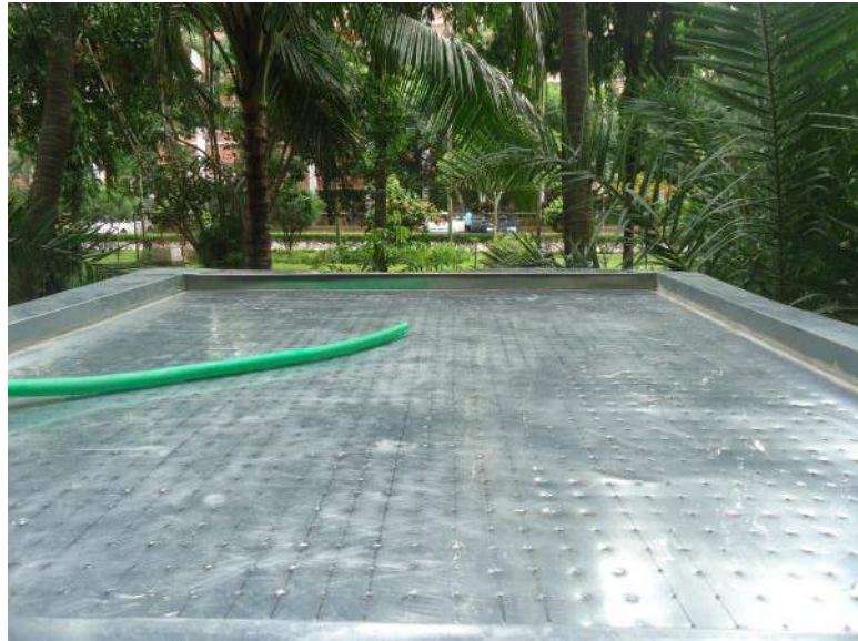
Figure 3.11: Perforated GI sheet for rainfall distribution
