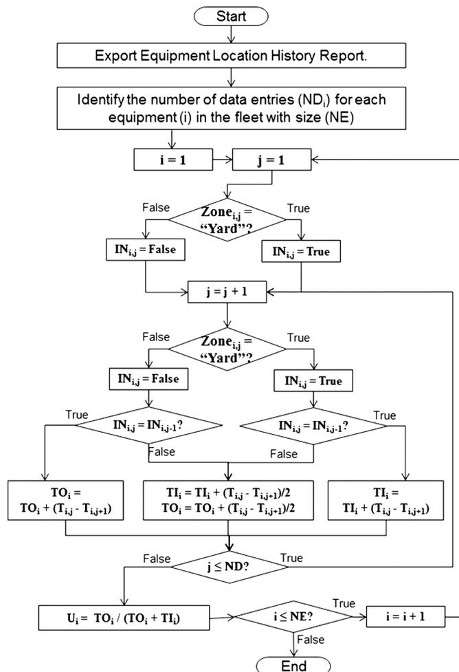
Fig. 5. Telematics-based fleet-use assessment algorithm
