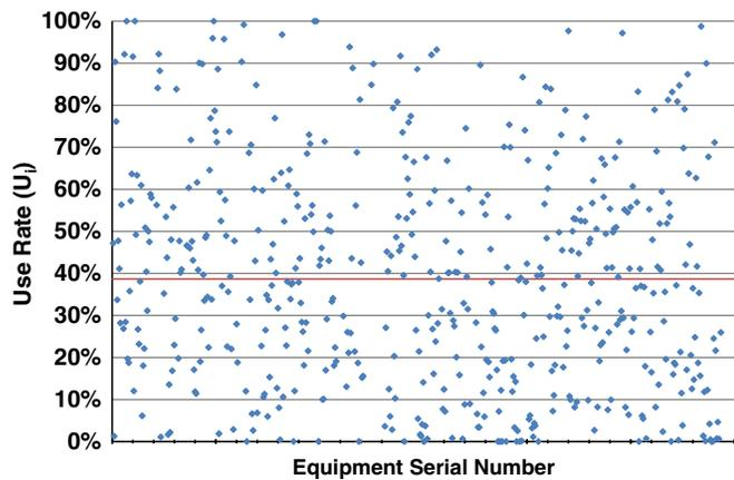
Fig. 6. Plot of equipment individual-use rates and average fleet-use rate
