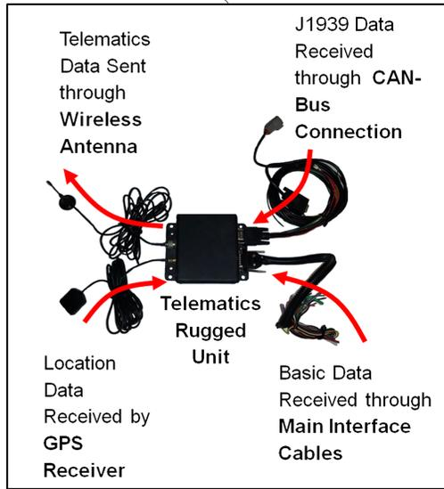
**Fig. 3.** Telematics transponder unit installation and connections (images courtesy of DPL America)
