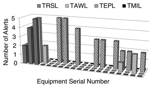
**Fig. 8.** Visualization of equipment health parameter (engine lamps) for dozers
