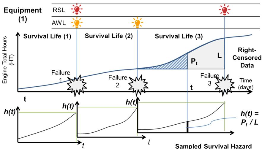
**Fig. 9.** Telematics-based sampling of equipment failure and survival lives
