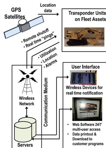
Fig. 1. Telematics system components and data flow
