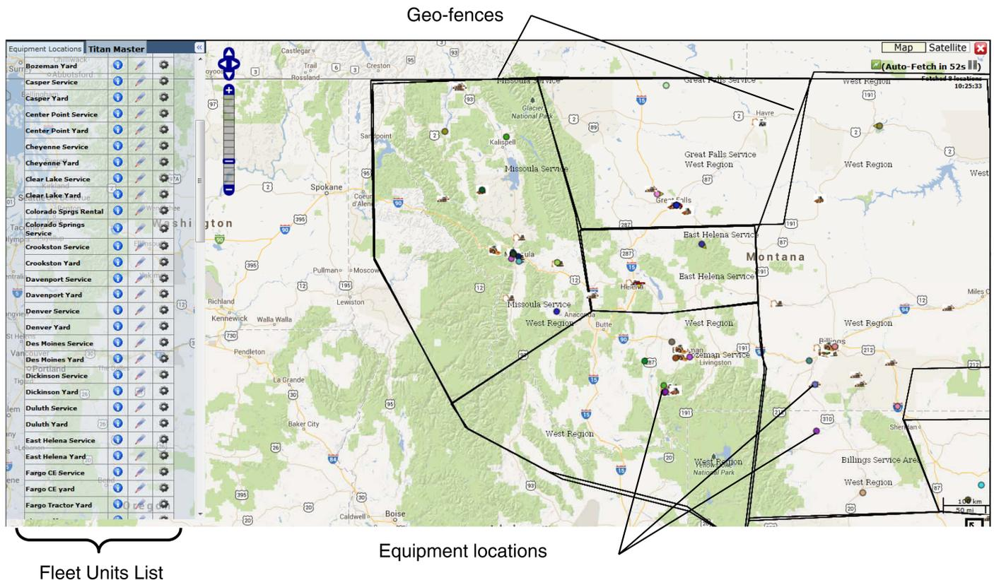
Fig. 2. Telematics user interface, locations map, and use of geo fences (image courtesy of DPL America)
