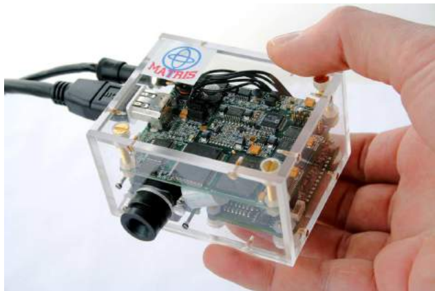
Figure 3: A hardware prototype of the MATRIS project, integrating a camera and an IMU in a single housing. It provides a hardware synchronised stream of video and inertial data.
