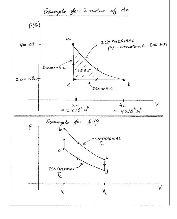
This is what an engine is supposed to do. A closed clockwise cycle will function as an engine. A closed counter-clockwise cycle will function as a refrigerator. For our engine cycle, a net  $Q_{in} = 553 + 598 = 1151$  Joules is transferred into the gas, and a net  $Q_{out} = 998$  Joules is transferred out of the gas. The difference  $W_{by} = Q_{in} - Q_{out}$  is the work done by the gas.
