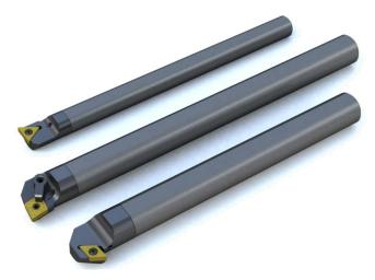
Boring tools consist of a round shaft with one insert pocket designed to reach into a part hole or cavity to remove internal stock. Boring tools enlarge a hole made by a previous process.
