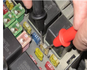
VOLTAGE DROP TESTING ACROSS FUSES
