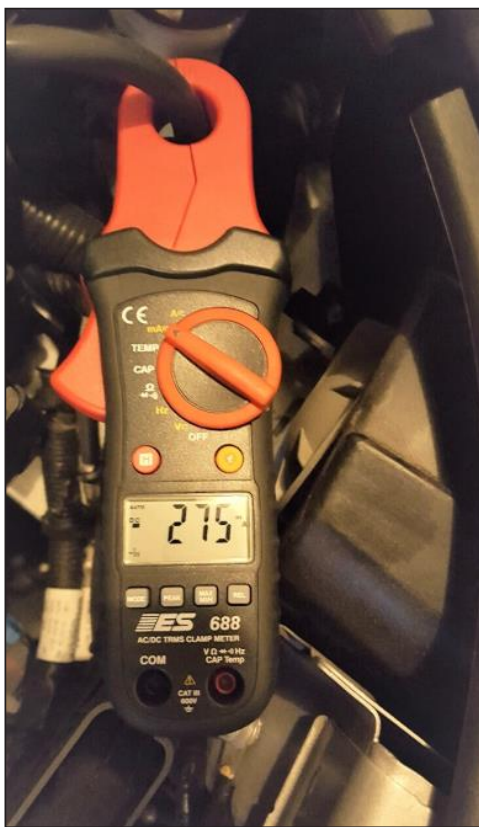
The inductive ammeter being used on a battery cable to measure parasitic draw results
