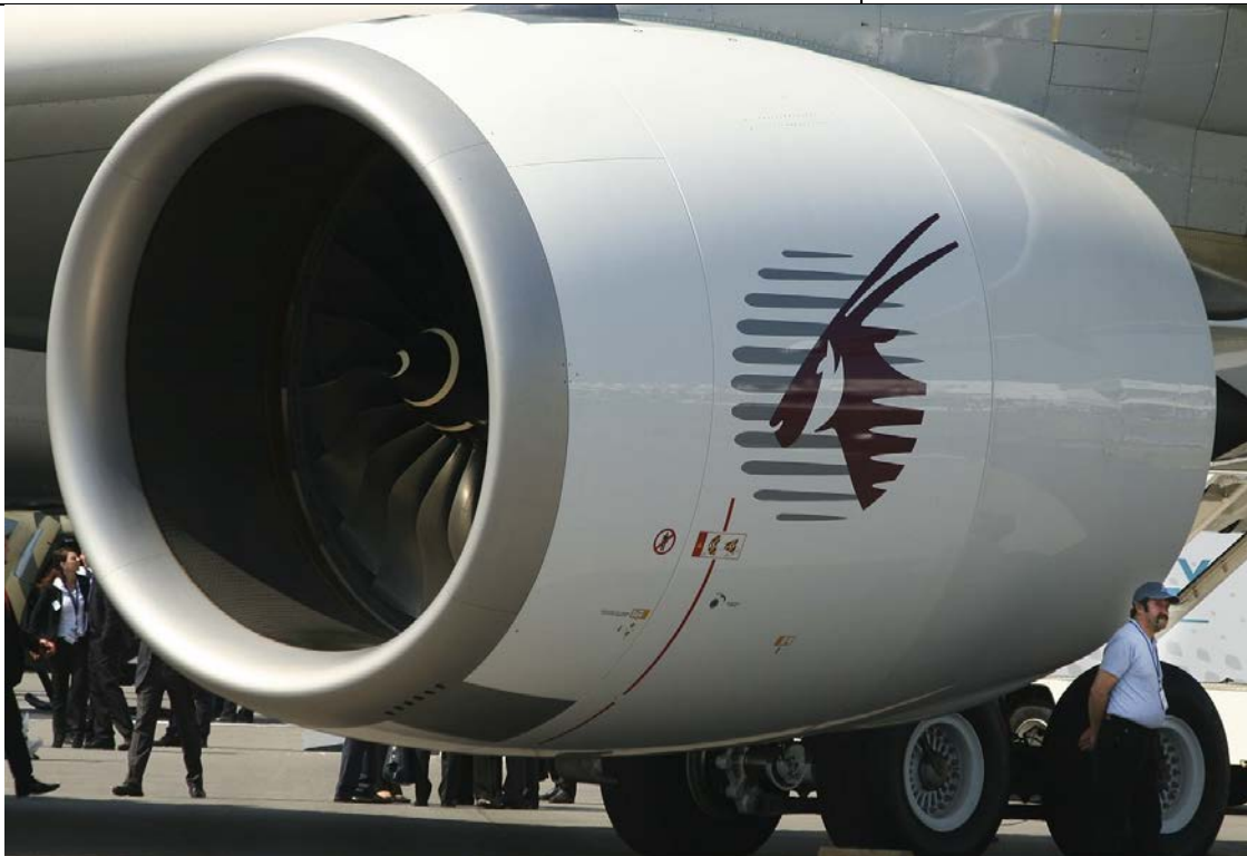
Rolls-Royce Trent XWB fanjet engine installed under the Airbus A350's wing (compare size to person lower right) 244
