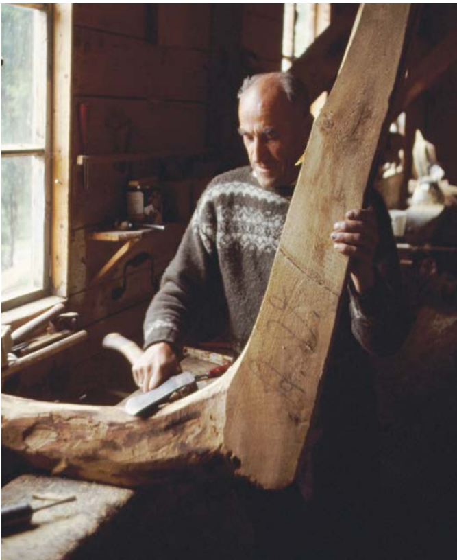
Source 1 A Norwegian shipbuilder carving a stern post (back) using the same methods his Viking ancestors did more than a thousand years ago
