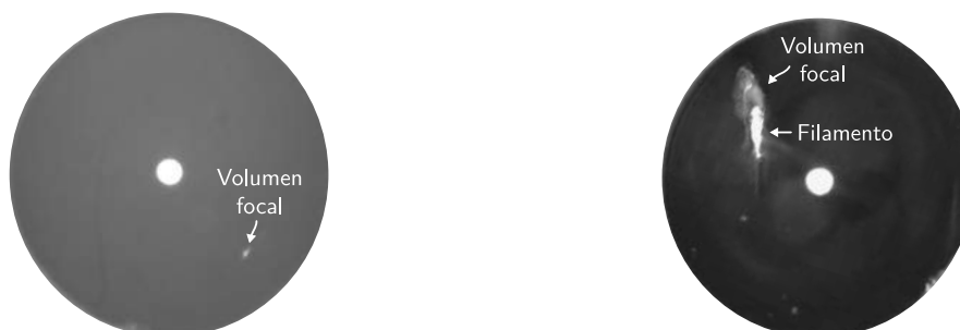
(a) Óptica adapt. ( E_p = 0.19 \mu\text{J} , PRR = 60 kHz) (b) Exp. directa ( E_p = 1.09 \mu\text{J} , PRR = 120 kHz)
