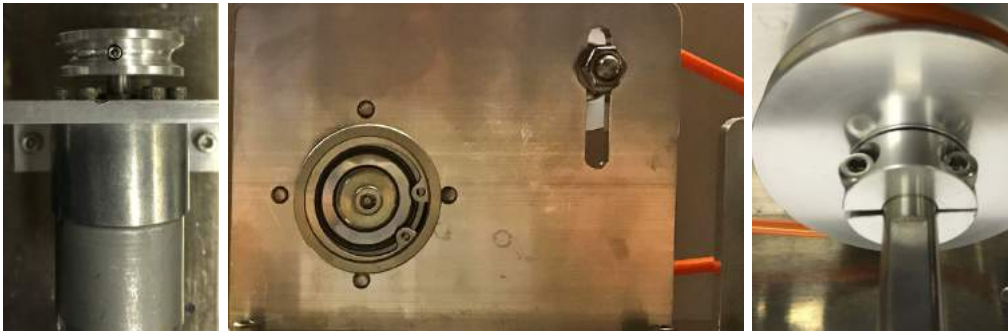
Figure 6. Close-up views of specific challenges in the 3D assembly problem. Left: (seen from above) the motor axis needed to be inserted into the mounting plate so that the six screw holes are aligned with the holes in the mounting plate. Note that the motor axis was not in the center of the motor case. Center: (seen from behind) inserting the ball bearing into the mounting plate required considerable force (tight fit), as well as alignment of four screw holes that are inserted from the other side. This close-up also shows the sliding mount for the pulley that stretches the rubber band. Right: To attach the pulley to the shaft, it had to be held in place while the two screws were fastened.
