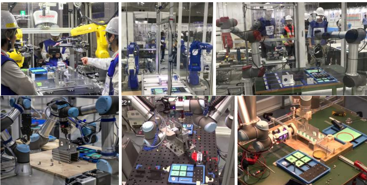
Figure 5. Sample solutions to the 3D assembly task from the teams FA.COM, JAKS, Robotic Materials (left to right, top), O2AS, SDU Robotics, Cambridge Robotics (bottom). The different solutions illustrate the drastically varying use of external sensors and utilities such as tool changers.
