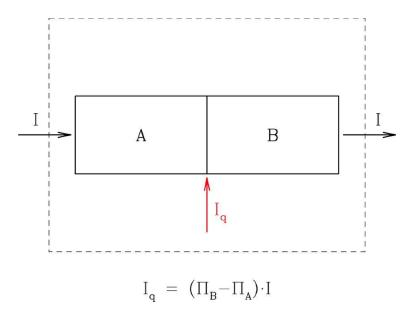
Figure 8.8: A sketch of a Peltier effect refrigerator. An electrical current I is passed through a junction between two dissimilar metals. If the dotted line represents the boundary of a thermally well-insulated body, then the body cools when  $\sqcap_{\rm B} > \sqcap_{\rm A}$ , in order to maintain a heat current balance at the junction.
