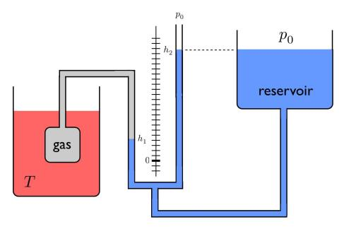
Figure 2.3: The constant volume gas thermometer. The gas is placed in thermal contact with an object of temperature T. An incompressible fluid of density  $\varrho$  is used to measure the pressure difference  $\Delta p = p_{\rm gas} - p_0$ .
