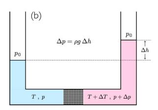
Figure 5.11: The fountain effect. In each case, a temperature gradient is maintained across a porous plug through which only superfluid can flow. This results in a pressure gradient which can result in a fountain or an elevated column in a U-tube.
