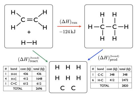
Figure 2.42: Calculation of reaction enthalpy for the hydrogenation of ethene (ethylene), C<sub>2</sub>H<sub>4</sub>.
