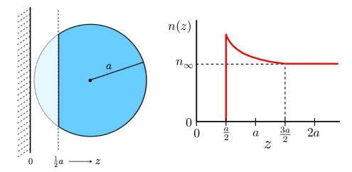
Figure 6.12: In the presence of a hard wall, the Mayer sphere is cut off on the side closest to the wall. The resulting density n(z) vanishes for  $z < \frac{1}{2}a$  since the center of each sphere must be at least one radius  $(\frac{1}{2}a)$  away from the wall. Between  $z = \frac{1}{2}a$  and  $z = \frac{3}{2}a$  there is a density *enhancement*. If the calculation were carried out to higher order, n(z) would exhibit damped spatial oscillations with wavelength  $\lambda \sim a$ .
