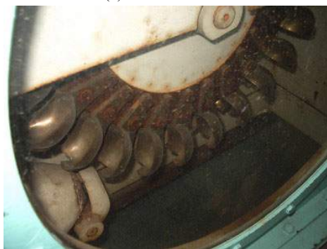
(c) Pelton wheel, including deflector vane
