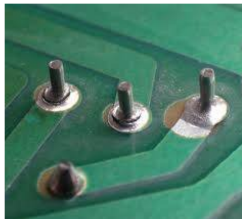
More "Dry Joints."
