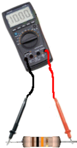
Fig 23. Resistance Measurement with a DMM
