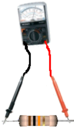
Fig 22. Resistance Measurement with Analogue Multimeter
