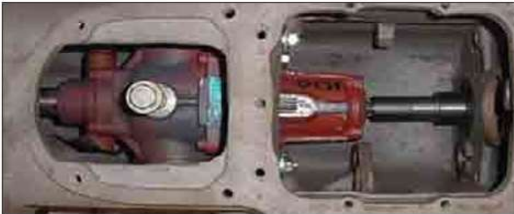
Hydrostatic transmission inside a tractor engine
