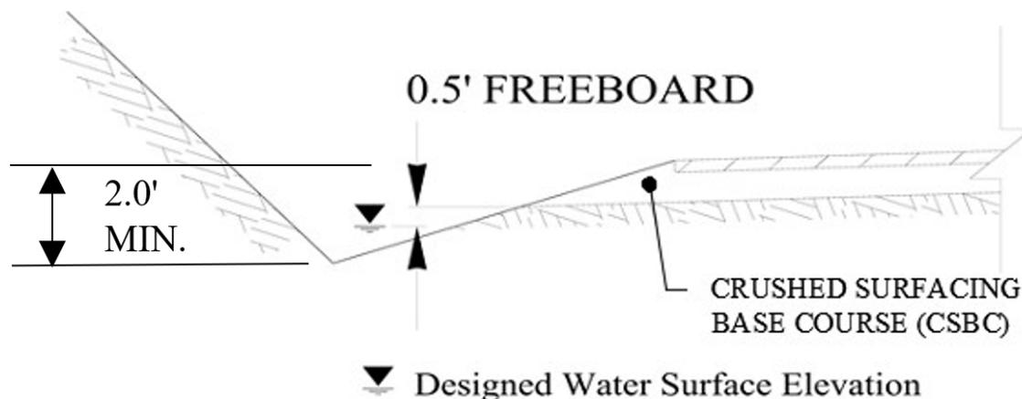
Ditches should not be confused with biofiltration swales. In addition to collecting and conveying drainage, biofiltration swales provide runoff treatment by filtering out sediment. (See the [Highway Runoff Manual](#) for design guidance for biofiltration swales.) Roadside ditches are to be designed so the integrity or geometry of the roadway is not compromised.
