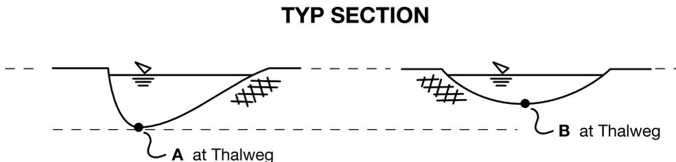
In both uniform and non-uniform channels, the engineer may need to apply discretion in how the gradient reaches are assessed and/or combined to best represent the channel hydraulic conditions, and where the thalweg is located.
