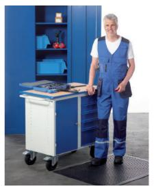
Tool trolleys can be used as a moving workstation. A rubber mat provides good support if you have to stand a lot.
