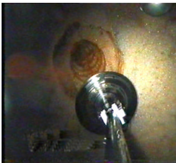
Fig. 14: Defoaming of a fermenting vessel
