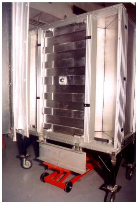
Fig. 12: Photograph of the rectangular plate transducer with reflectors
