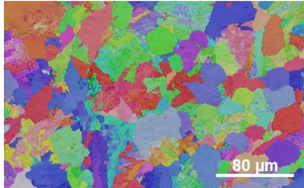
Fig.4.7 Typical orientation and size of the grains in the investigated steel grades.
