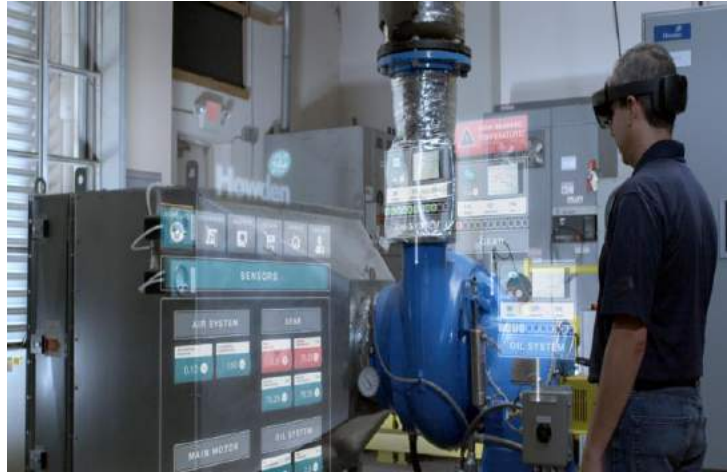
Figure 1.16 - Using Vuforia Studio to Understand Equipment
