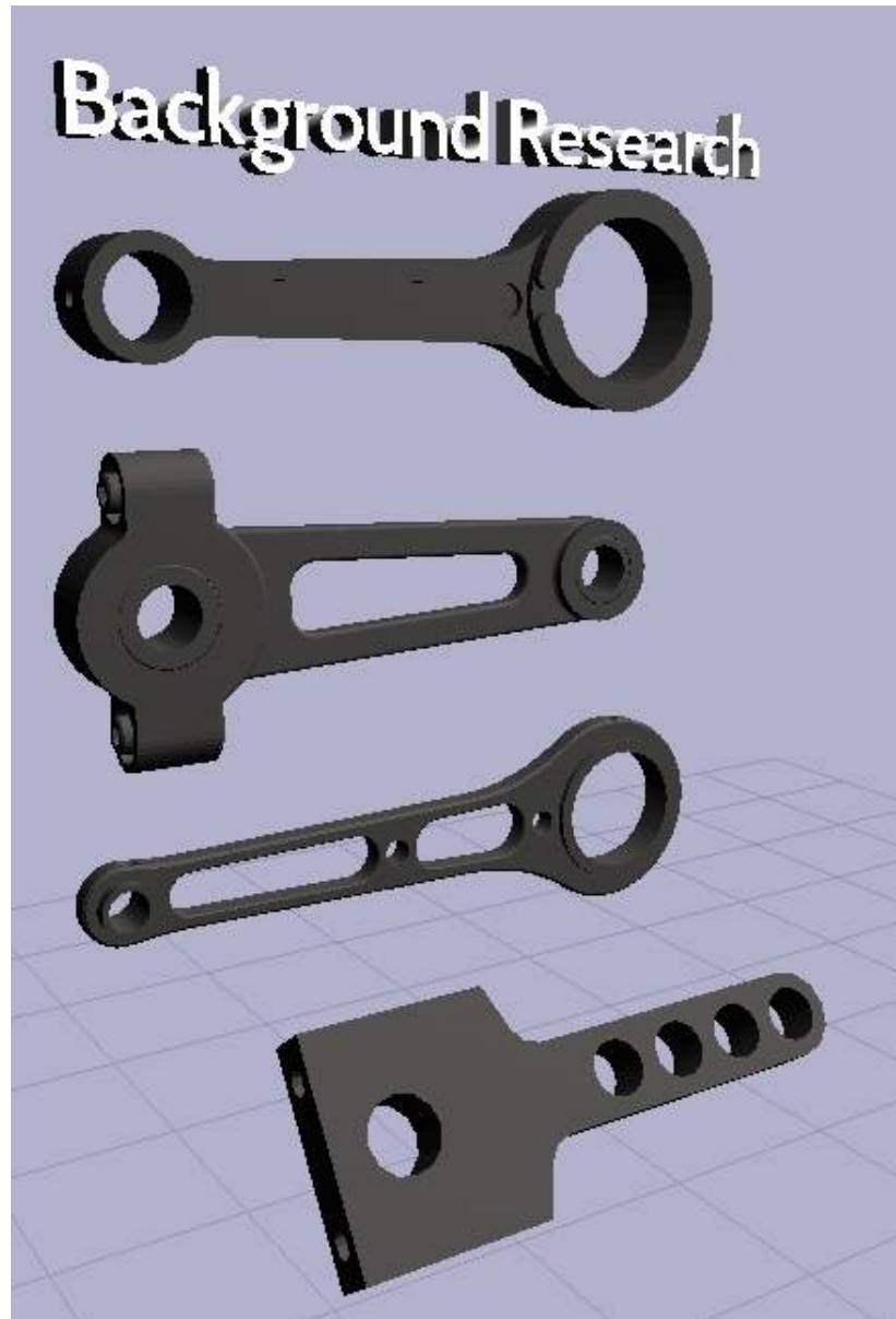
Figure 3.4 - Various Connecting Rod Designs Viewed in VR
