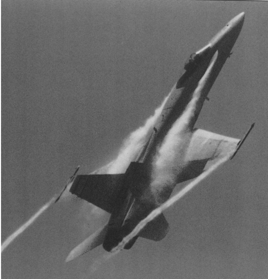
Figure 3.19: Vortex Flows on an F-18 (NASA Photo)
