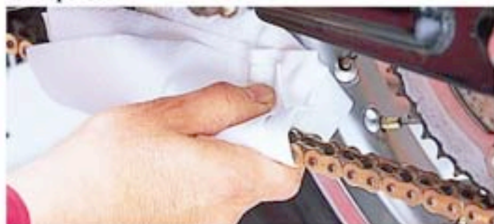
Wipe the solvent cleaner on each links.
