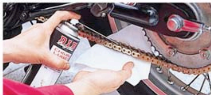
Lubricating each links and parts of seal.
