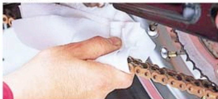
1:Rotate the chain wheel for accustoming chain links and sprokets. 2:Remove the excess oil.
