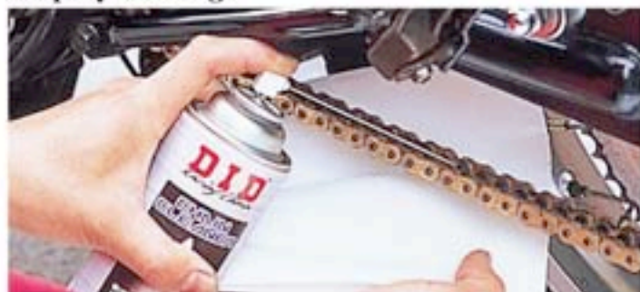
1:Set the tray under the chain. 2:spray the chain cleaner.
