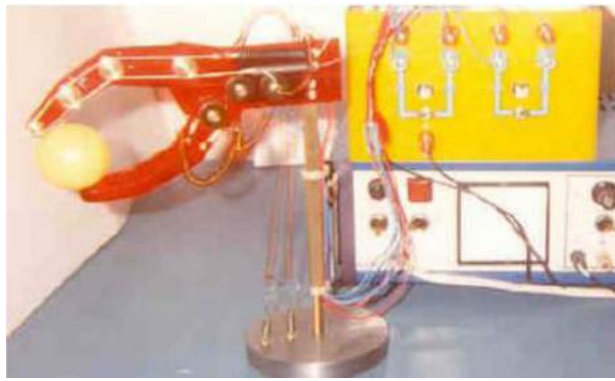
Figure 19 An artificial hand prosthetic device using SMA wires (see online version for colours)
