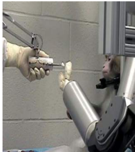
Figure 2 In this successful experiment, collected signals from monkey's cortex were used by it to control a robotic arm and feed itself using it (see http://en.wikipedia.org/wiki/Brain%E2%80%93computer_interface ) (see online version for colours)
