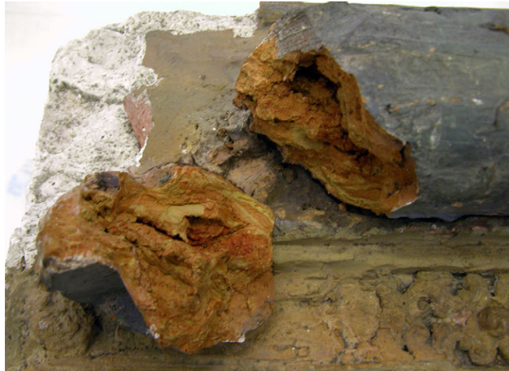
Figure 3. Detail showing the different veins of colour present in the clay blocks indicating that the clay mixture was not well blended. © IMC-DGPC
