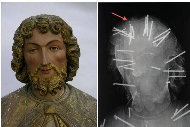
Figure 4. Joseph with Child. Studio Thissen, 1884. Petruskerk, Venray. The nails used to hold the carved wooden support together are visible in the X-radiograph. The arrow (red) indicates a putty filler used to cover the nail head. ©SRAL
