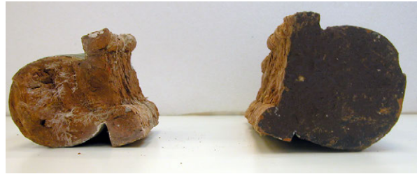
Figure 2. Detail of two sections of the broken column and the mastic putty. © IMC-DGPC
