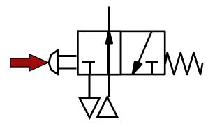
The valve symbol can be visualised as moving to align one state or another with the port connections
