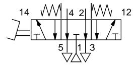
Treadle actuated, detented, all ports sealed centre
