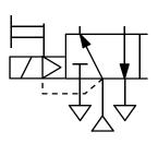
When no integral or external pilot supply is shown it is assumed to be integral
