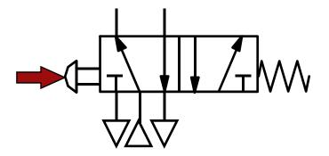
The full symbol is then made by joining the two boxes and adding operators. The connections are shown against only the prevailing state
