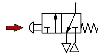
The valve symbol can be visualised as moving to align one state or another with the port connections
