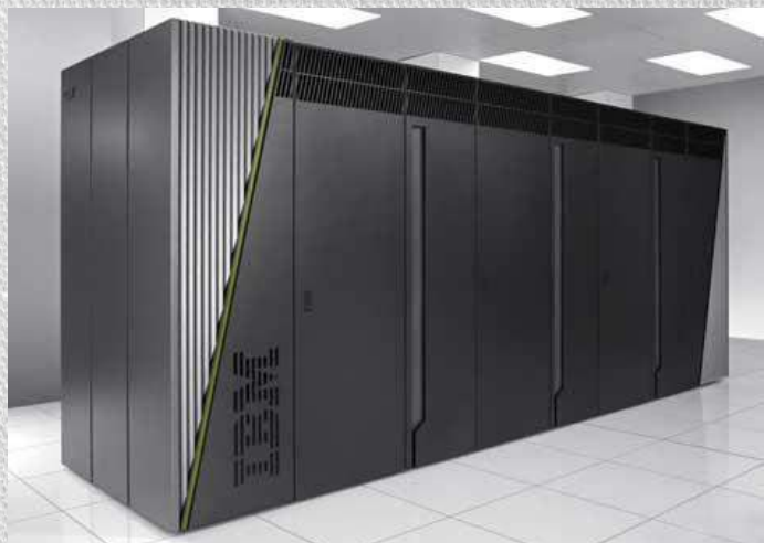
IBM Blue Gene / Q systems powering the Fermi supercomputer at Cineca in Italy.
