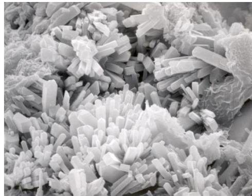
**Figure 3.-** SEM photo of *prismatic phillipsite crystals from the "Yellow Neapolitan Tuff".*
