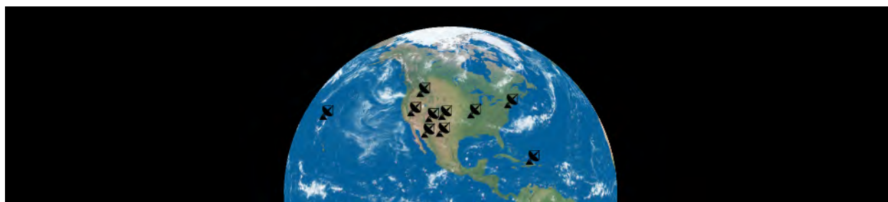
Figure 6.21 Very Long Baseline Array. This map shows the distribution of 10 antennas that constitute an array of radio telescopes stretching across the United States and its territories.
