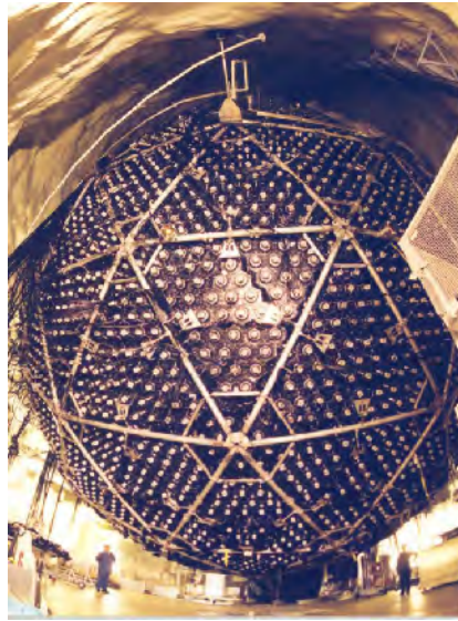
Figure 16.20 Sudbury Neutrino Detector. The 12-meter sphere of the Sudbury Neutrino Detector lies more than 2 kilometers underground and holds 1000 metric tons of heavy water. (credit: A.B. McDonald (Queen's University) et al., The Sudbury Neutrino Observatory Institute)
