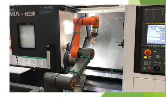
Machine Loading Robot
