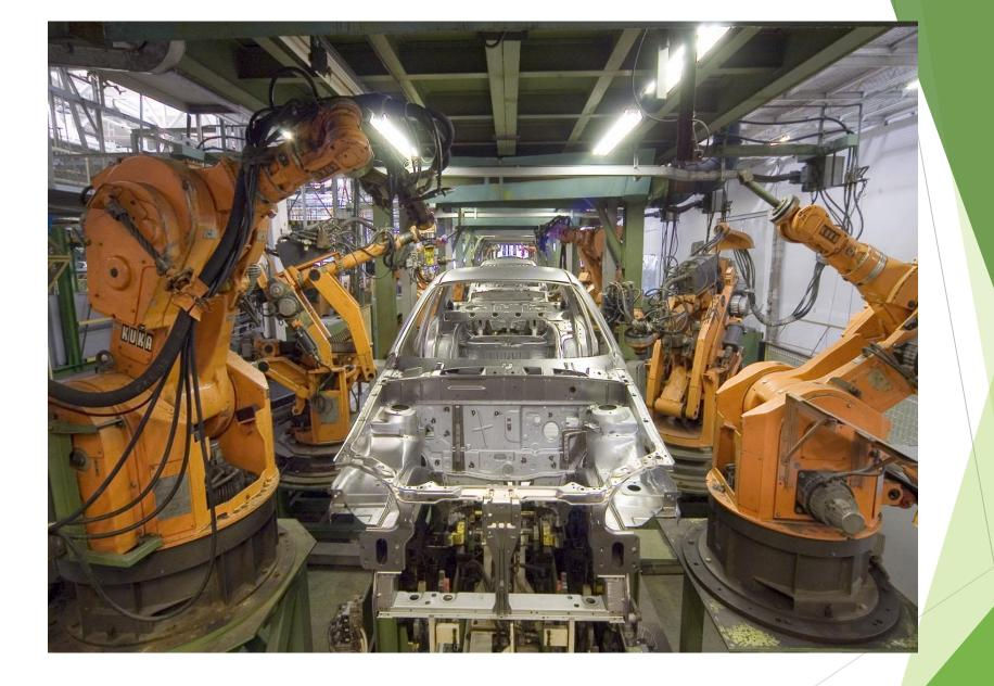
Industrial Robots being used for Automotive Manufacturing And Assembly
