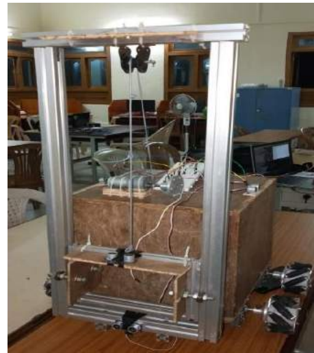
Fig. 10. Prototype of Autonomous wall painting robot
