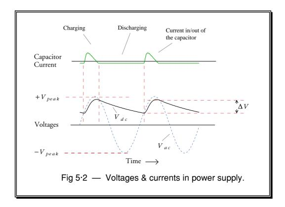
The input transformer 'steps down' the mains input to provide a 50Hz sinewave voltage<sup>1</sup>,  $V_{ac}$ , which swings up & down over the range  $+V_{peak}$  to  $-V_{peak}$  as shown in figure 5.2. The value of  $V_{peak}$  depends on the turns ratio of the transformer. The voltage on the capacitor,  $V_{dc}$ , at any moment depends on how much charge it holds.
