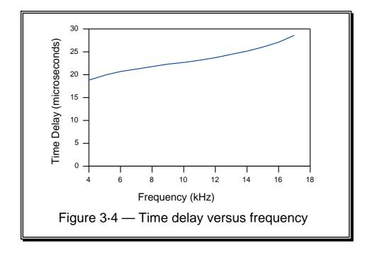
Looking at figure 3.4, we can see that when expressed in terms of a time, the delay seems rather more uniform and does not vary as quickly with frequency as does the phase. This behaviour is
