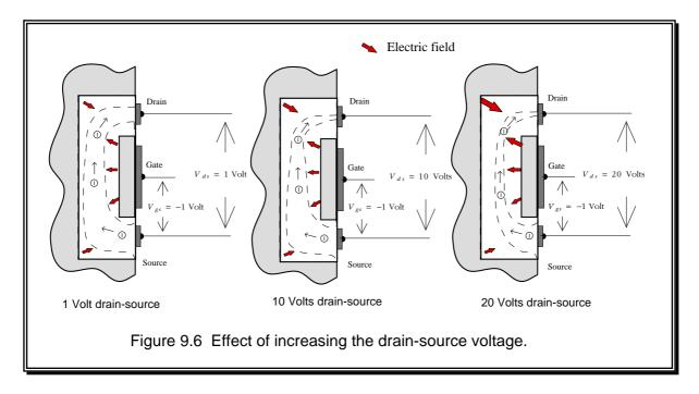
With a steady gate-source voltage of -1 V there is always 1 volt across the wall of the channel at the source end. A drain-source voltage of 1V means that there will be  $\underline{2}$  volts across the wall at the drain end. (The drain is 'up' 1V from the source potential and the gate is 1V 'down', hence the total difference is 2V.) The higher voltage difference at the drain end means that the electron channel is squeezed down a bit more at this end.
