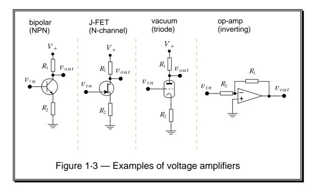
Figure 1.3 shows four examples of simple voltage amplifier stages using various types of device. In each case the a.c. voltage gain will usually be approximated by
