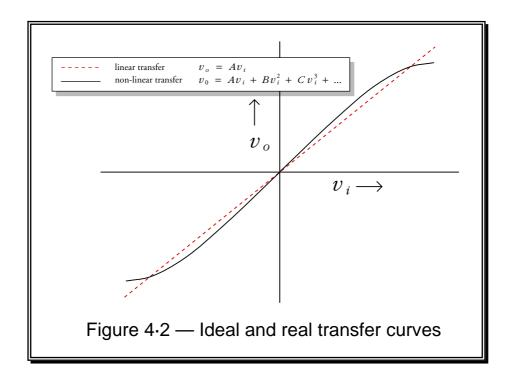
The term *Distortion* is usually used to mean that the amplifier has a gain which depends upon the signal amplitude (or sometimes also the frequency). The effect is described as an effect which arises due to *non-linearity*. Figure 4-2 illustrates the kind of non-linearity we are concerned with here. We can distinguish an ideal amplifier from a realistic one in terms of the *Transfer Curve* – the plot of  $v_0$  versus  $v_i$  – and the expressions that relate the input to the output.
