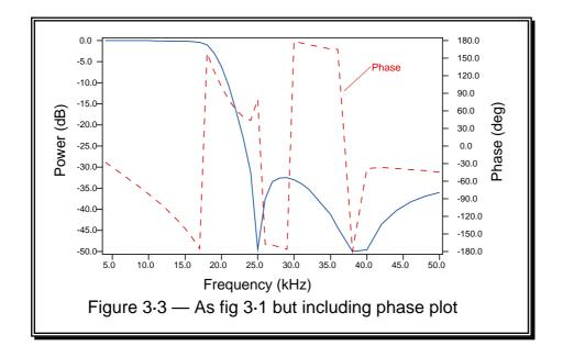
Although a frequency response of the kind shown in figure 3.1 is the most common way to display the behaviour of a filter, it doesn't tell the whole story. When sinewave components pass through the filter they may also be delayed by an amount that depends upon their frequency.
