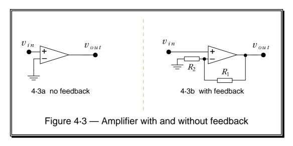
Figure 4.3 shows the amplifier in two situations. 4.3a shows the amplifier with no applied feedback. 4.3b shows a modified circuit where a pair of resistors applies feedback to the non-inverting input of the amplifier. This feedback is subtracted from the actual input and tends to reduce the signal levels, hence it is conventionally called *Negative Feedback*.
