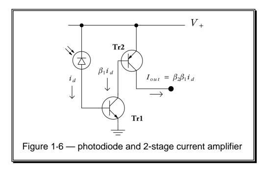
Figure 1.6 shows an example of a 2-stage current amplifier in a typical application. The photodiodes often used to detect light tend to work by absorbing photons and releasing free charge carriers. We can then apply a potential difference across the photodiode's junction and 'sweep out' these charges to obtain a current proportional to the number of photons per second
