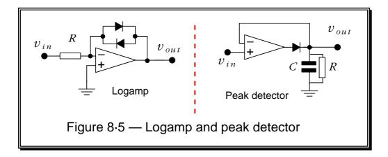
Figure 8.5 shows two examples of circuits which combine an Op-Amp with diodes to perform some useful non-linear function. The logamp exploits the fact that the effective resistance V / I of a diode varies with the applied voltage. For a 'textbook' diode we can say that the current and voltage will be linked via an expression of the form
