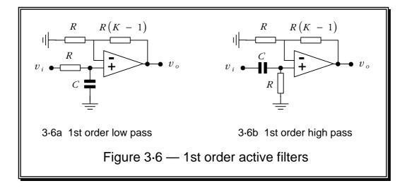
Figure 3.6 shows 1st order low and high pass active filters. For a Normalised version we would assume that  $R = 1\Omega$  and C = 1F. More generally we can say that the frequency response of  $A_v$ for each of these will have the form
