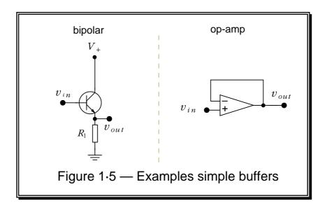
Figure 1.5 shows two simple examples of buffers. In each case the gain device (an NPN transistor or an op-amp in these examples) is used to lighten the current load on the initial signal source that supplies  $v_{in}$ . An alternative way to view the buffer is to see it as making the load impedance seem larger as it now only has to supply a small current to ensure that a given voltage is output.
