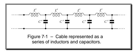
The amount of capacitance/metre and inductance/metre depends mainly upon the size and shape of the conductors. The inductance relates the amount of energy stored in the magnetic field around the cable to the current level. The capacitance relates the amount of energy stored in the electric field to the potential difference between the conductors. For co-ax and twin feeders the values are given by the expressions in the table below, where the relevant dimensions are as indicated in figure 7.2.
