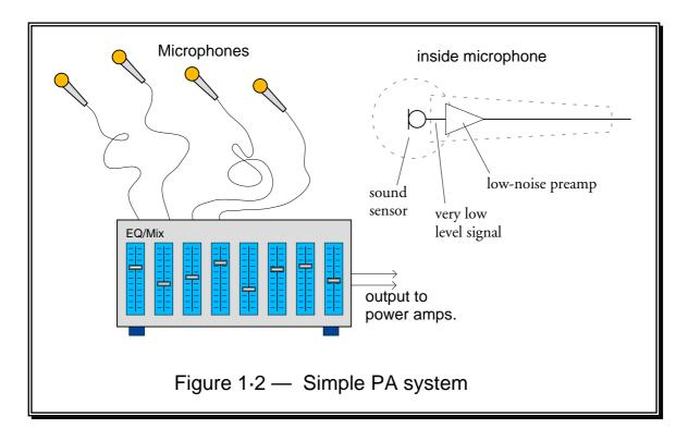
The system shown in figure 1.2 is similar to the previous arrangement, but in this case is used for taking signals from microphones and 'mixing' them together to produce a combined output for power amplification. This system also include an 'EQ' unit (Equalising) which is used to adjust and control the frequency response.
