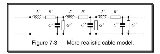
Here the dissipative loss due to conductor resistance is indicated by a resistance-per-length value of R' and loss due to the dielectric is represented by a conductance-per-length value of G'. As before, here I have used primes to emphasise that the values are per unit length and avoid confusion with total values or those of specific components.
