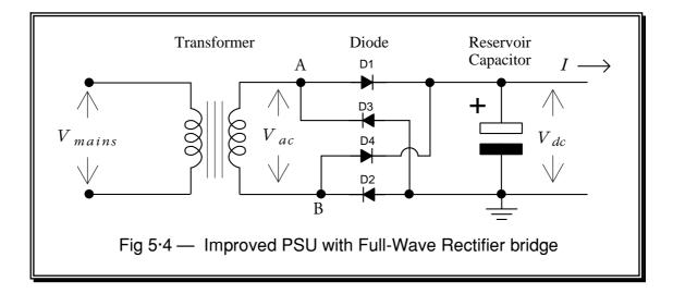
As with the simple arrangement, the reservoir capacitor is charged whenever the input a.c. is large enough. However this can now happen in two ways which we can understand by considering the relative voltages,  $V_A$  and  $V_B$  at the two points, 'A' and 'B' shown on figure 5.4
