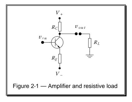
The amplifier is supplied via power lines at  $V_+$  and  $V_-$  so we can immediately expect that this will limit the possible range of the output to  $V_+ > v_{out} > V_-$  as the circuit has no way to provide voltages outside this range. In fact, the output may well be rather more restricted than this as we can see using the following argument.
