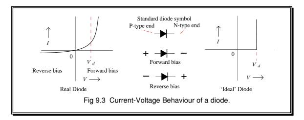
The polarity which produces a significant current is called *Forward bias*. When we raise the forward bias voltage we reduce the diode's energy barrier. This essentially reduces the diode's resistance. We might therefore expect it's effective resistance to vary approximately  $\propto 1/V_f$ . i.e. we can say that the diode's effective resistance at a given forward voltage will obey an equation like
