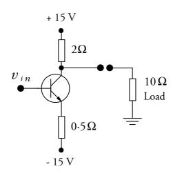
Q2) The diagram on the left shows a single ended Class A amplifier output stage. What are the values of the maximum positive and negative voltage the amplifier can apply to the load resistor? How much power does the amplifier dissipate when providing no output? What is the mean value of the maximum undistorted sinewave power level the amplifier can supply to the load? [max +ve +12.5V. most -ve -8.65 V, quiescent dissipation 225 W, 3.75 W]
