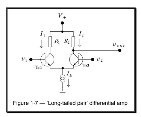
This particular example uses a *Long-Tailed Pair* connected to a *Current Source*. We can understand how the circuit works simply from an argument based upon symmetry. For simplicity in this diagram we represent the Current Source by the standard symbol of a pair of linked circles. We will look at how a current source actually works later on. For now we can just assume it is an arrangement that insists upon always drawing a fixed current which in this case has the value  $I_E$ .
