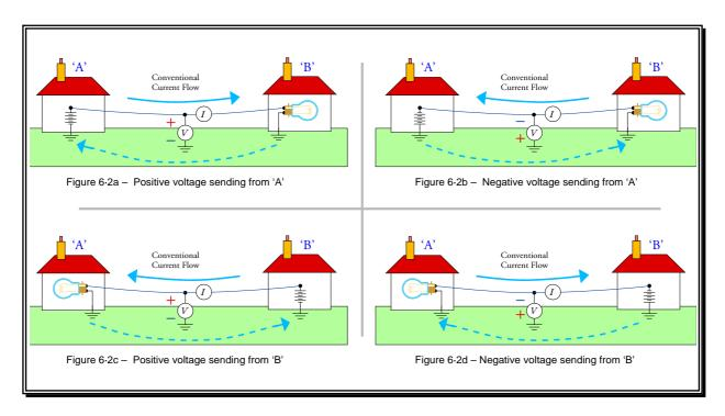
The results obtained by observing the meters in each case can be listed as follows if we define a flow of conventional current from  $A \to B$  as having a positive sign we can draw up the following table of results.
