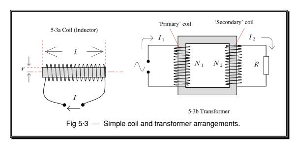
The basic properties of a *transformer* can be explained in terms of the behaviour of *inductors*. Figure 5.3a shows a coil of wire wound around a rod. Passing a current along the wire will produce a magnetic field through & around the coil. This current-field relationship works both ways — i.e. applying a magnetic field through the coil will produce a current. By looking at a good book on electromagnetics we can find the relationship
