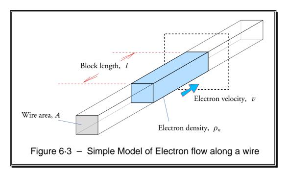
Here we imagine the 'free' electrons that can provide the moving charges that constitute the current as having a uniform number density inside the material of  $\rho_n$  electrons per unit volume. The current is the result of these moving along the wire at an average velocity, v. We can now define the current to be
