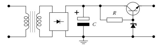
The transformer provides an an output a.c. voltage to the full-wave diode bridge of 20 Volts rms at a frequency of 50Hz. What will be the value of the peak voltage supplied to the reservoir capacitor, C? [27 Volts]
