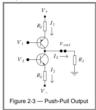
The circuit shown on the left now has two transistors which we can control using a pair of input voltages,  $V_1$  and  $V_2$ . We can therefore alter the two currents,  $I_1$  and  $I_2$  independently if we wish.
