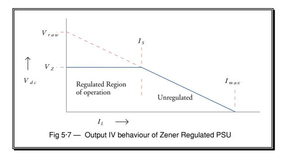
We can divide the operation into two areas – regulated and unregulated. In the regulated area the output voltage is controlled by the action of the Zener, and in the unregulated region it is not. In the regulated region we have
