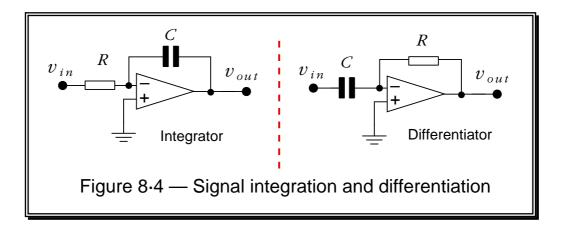
Figure 8.4 shows a pair of circuits which we can use to integrate or differentiate a signal value with respect to time. The *Integrator* acts to provide an output level proportional to the time-integral of the input level. It provides an output voltage at a time,  $t_1$  given by
