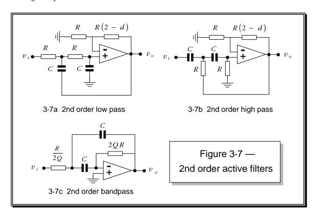
In this case an example of a band-pass filter is also included. The examples shown introduce two new quantities that have standard definitions. The *Damping* value, d, and the *Quality* factor, Q The gain value, K is related to these via the expressions
