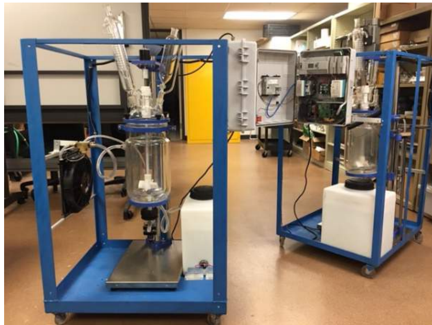
Figure 3: Bioreactors 2 and 3 with PLC based automation
