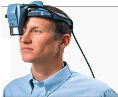
Figure 5: Virtual Retinal System HMD.
