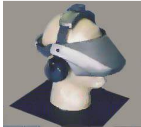
Figure 7: Video See-Through HMD.
