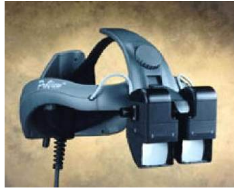
Figure 2: Optical See-Through HMD.
