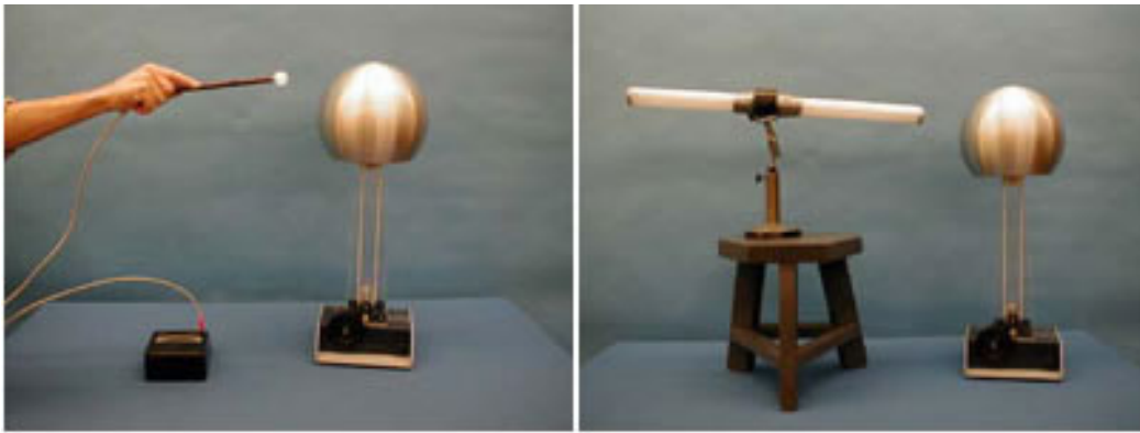
Figure 15: A voltmeter and a fluorescent bulb make manifest the existence of a potential difference (and electric field).
