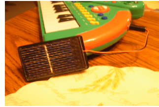
Figure 85: Demo. A transformer is used to modulate, that is to change the intensity, of a laser following an audio input. The variations in the intensity of the light are detected by a solar cell (or photoelectric panel) and converted into sound by an amplifier. The same principle works if we use a LED but the laser beam stay narrow at much longer distances and transmits the signal more effectively.
