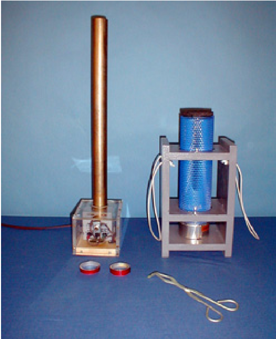
Figure 63: Demo. Starting up the current through the coil induces a current on a ring producing a repulsive force and shooting the ring in the air. Cooling the ring decreases the resistance therefore increasing the induced current and the height reached by the ring.
