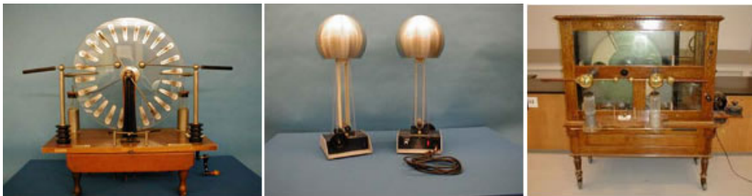
Figure 6: Machines used to generate static electricity. The first and last one are Wimshurst machines. In the middle is a small Van der Graaf generator. Van der Graaf made huge generators to accelerate atomic particles which can still be seen in the Boston museum of Science.
