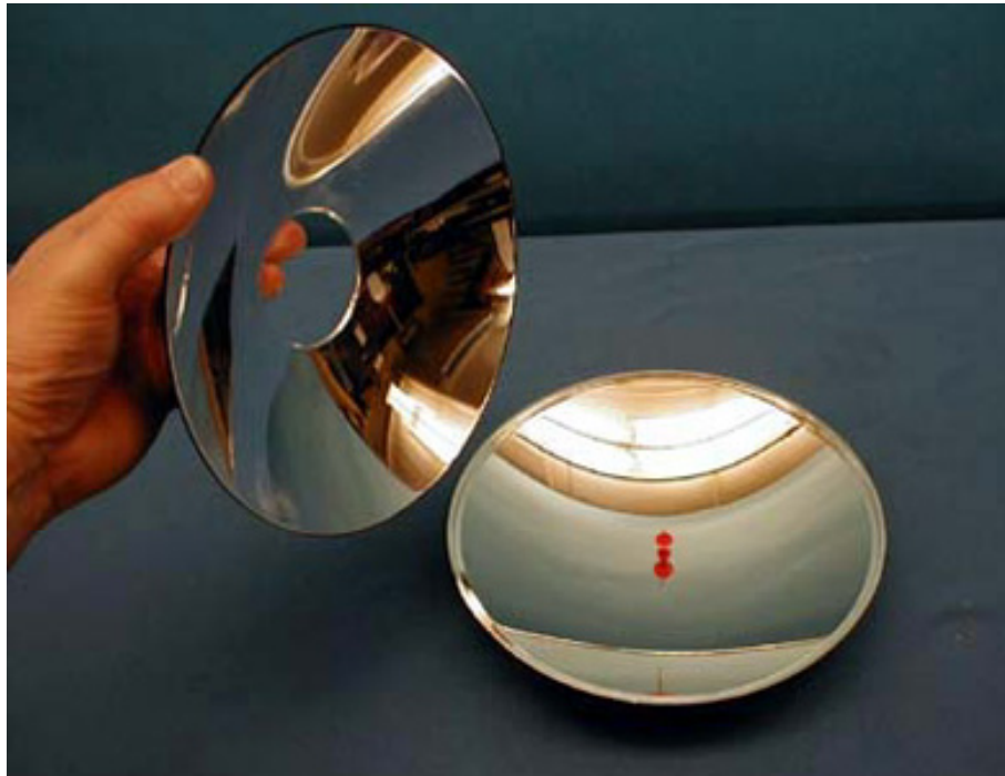
Figure 97: Demo: an interesting effect of real images. The image of a small object can be easily confused with the real thing.
