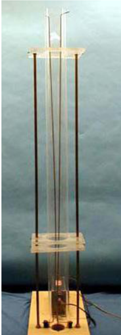
Figure 67: Demo. A transformer can be used to increase the voltage of an oscillating (alternate) current. The increased voltage can be used to create an interesting display.
