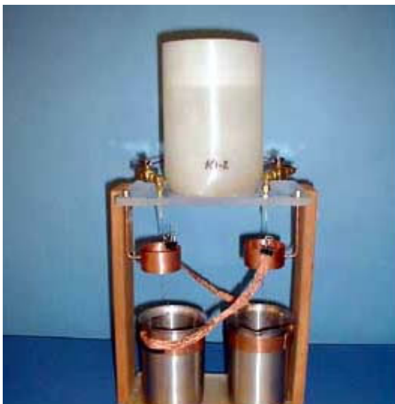
Figure 13: Kelvin invented this device to generate electricity. I find it of great interest since it is basically just water dropping from a tank and nevertheless it is able to generate electricity enough to light a few neon bulbs. Essentially illustrates how, by understanding how nature works one can create something interesting out of almost nothing.
