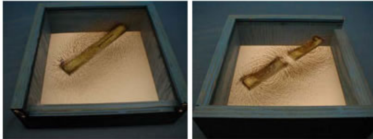
Figure 48: The lines of magnetic field can be made evident using iron filings which orient themselves parallel to the magnetic field.
