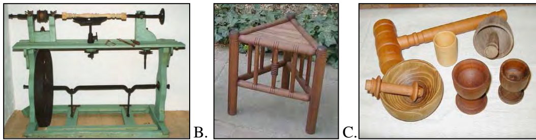
Figure 3. a) Lathe continuous rotary motion bearing burin (Archive of Samian Folklore, 2008), b), c) Furniture and objects which required turning for their construction
