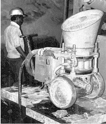
Typical dry mix shotcrete machine.
