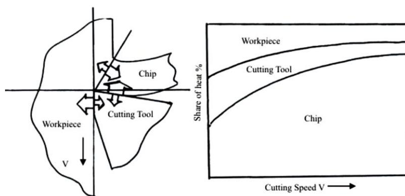
**Figure 2 Apportionment of heat amongst chip, tool and work piece (Rao, 2002)**
