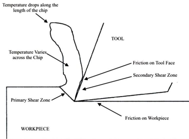
**Figure 1 Heat generated by chip formation (Trent et al, 1989)**
