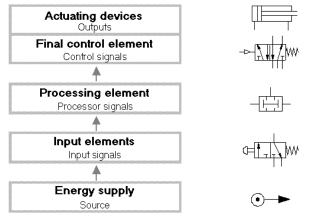
Pneumatic system structure and signal flow
