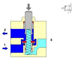
3/2 way valve, disc seat normally closed
