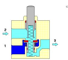
3/2 way valve, disc seat normally closed
