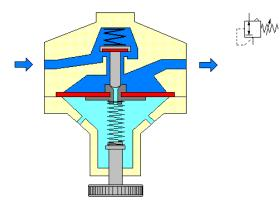
Air supply: Pressure regulator with vent hole
