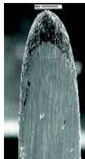
Fig 60: Diseño de la punta de Lima Liberator. (Tomado de Hilt, B.R., Cunningham, C.J., Shen, C., Richards, N. Torsional properties of stainless steel and nickel-titanium files after multiple autoclave sterilizations. J of Endod 2000; Vol. 26 No. 2 ) 31
