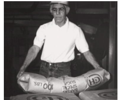
Manually lifting heavy, bulky load with no handles
