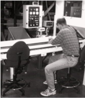
Control panels are too far from the worker.
