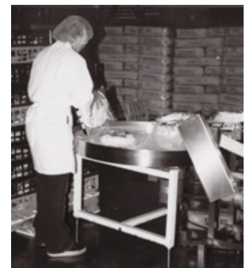
A raised work surface allows the worker to work in a more upright posture.
