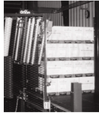
Automated shrink wrap equipment eliminates the need for workers to be in awkward postures.
