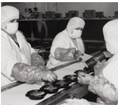
Squeezing liquid food product dispenser involves repetitive gripping with forceful exertions.
