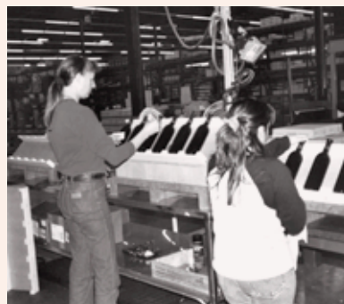
The addition or removal of a platform allows the height of the work surface to be adjusted to fit each worker.
