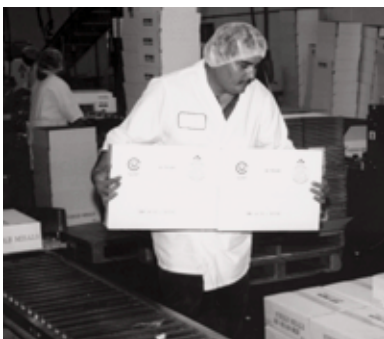
Manually lifting heavy, bulky load with no handles
