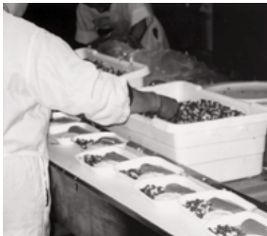
A worker must reach across the conveyor to get access to the food bin.
