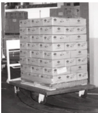
This pallet truck runs throughout the plant on a track.
