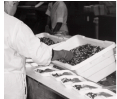
A tilted food bin allows the worker to reduce the reach into the bin.
