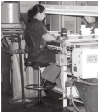
Adjustable chairs will allow workers to find the best seat height for them and their tasks.
