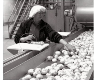
Extended reaches across a wide conveyor
