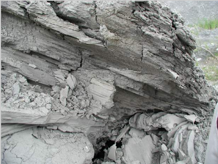
Fig. 1.15. Glaciolacustrine sediments of the former Lac du Trièves (image shows an approximate 1.5 m section).
