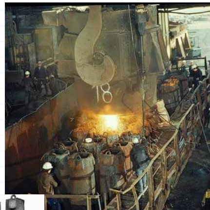
Teeming ingots at a steel mill
