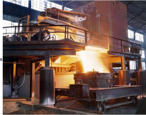
White-hot steel pours like water from a 35-ton electric furnace into a small ladle car. The transformer vault can be seen at the right side of the picture. For scale, note the operator standing on the platform at upper left. This is a 1941-era photograph and so does not have the extensive dust collection system that a modern installation would have, nor is the operator wearing a hard hat or dust mask
