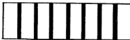
Fig. 2.7. Interference fringes on a flat surface viewed under an optical flat in a parallel beam of monochromatic light.
